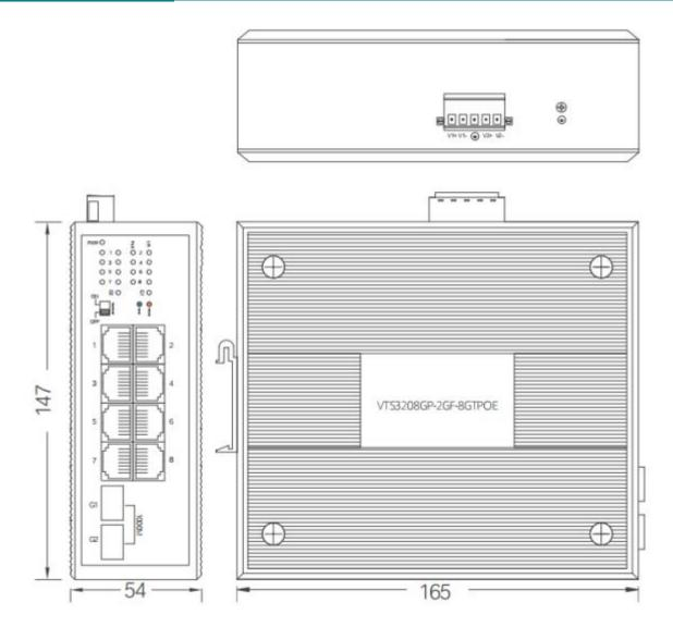
Din-rail mounting (Unit: mm)
