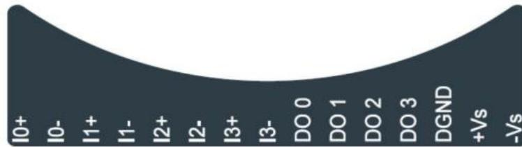
Figure 2.3 WISE-4010/LAN Pin Assignment
