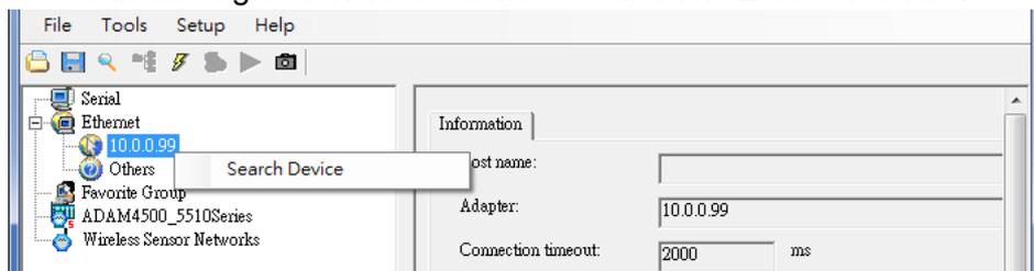
4. After the module been found, it will be listed under IP address in same domain, you can login the embedded web configuration web page for further configuration as introduced in previous section
