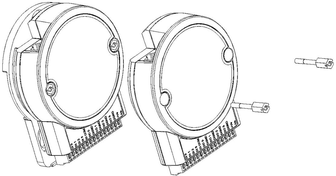
Figure 3.8 Stack Mounting
