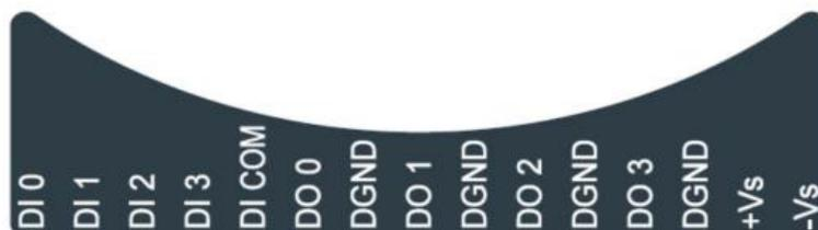
Figure 2.20 WISE-4050 Pin Assignment
