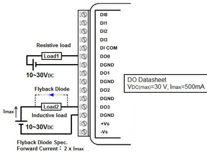
Figure 2.19 WISE-4050 Digital Output Wiring Diagram
