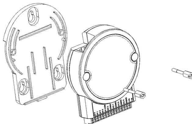
Figure 3.2 Installing the Mounting Kit for a DIN-Rail
